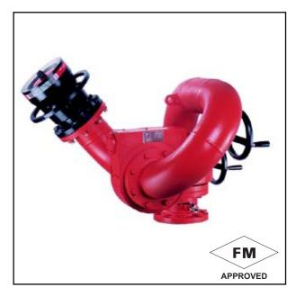
The monitor has welded carbon steel 6 inch (150 NB) water way. All steel parts are hot dip galvanized and epoxy painted for excellent corrosion resistance. The vertical and horizontal rotation is through corrosion resistant bronze swiveling joints with double row of stainless steel ball bearing. Both vertical and horizontal movements are controlled with handwheel driven fully enclosed worm gears and protected from the elements.
